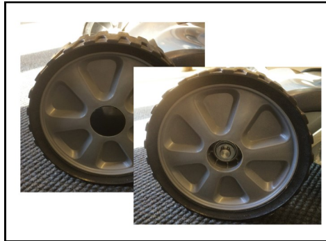
REMOVE WHEEL DUST COVER
